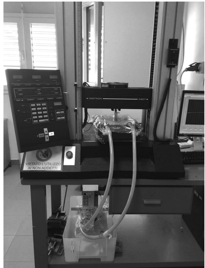
Figure 2. Hydraulic circuit to keep the temperature constant.
